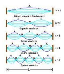
$$\psi(x,t) = Asen(kx - \omega t) + Asen(kx + \omega t) \tag{1}$$
